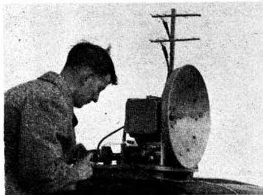
Mr. J. Spragg, G3APY, seen operating the combined 3 and 23 cm. equipment which helped bring the world's amateur 3 cm. record to the United Kingdom. On October 22, 1950, with the gear mounted atop of a saloon car, G3APY/P made two-way contact with G3ENS/P over a distance of 27 miles. Separate 5-element Yagi aerials are used for transmission and reception on 23 cm. with a wave-guide fed dipole and 18in. parabolic reflector on 3 cm.
